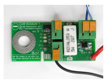
Bottom Cell Module's "RX+" and "RX-" signals should be connected via twisted pair to Control Unit's "CELL RX+" and "CELL RX-" wires correspondingly. It is
