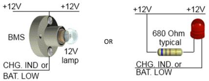
Lamp's one terminal or LED's "-" side must be connected to EMUS BMS Control Unit's output. Other lamp's terminal or LED's "+" side must be connected to +12V external power source. The source could be the same as supplying the power to BMS.
